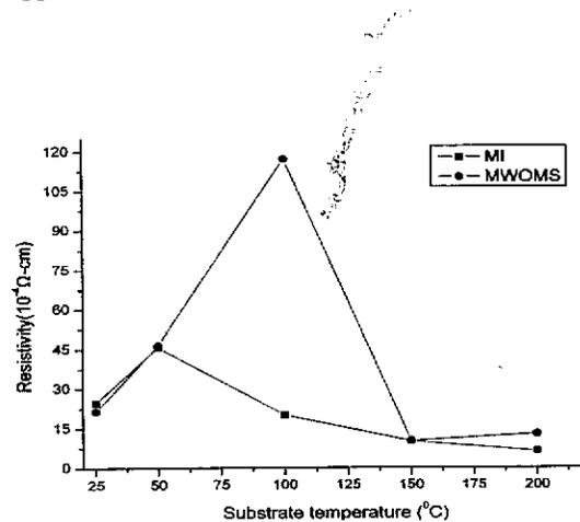
Fig.1. The electric resistivity of AZO films prepared with different substrate temperature was measured immediately (MI) and with one month storage (MWOMS) respectively after films production.
