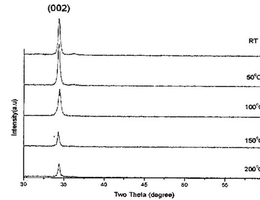
Fig.2. The X-ray diffraction spectra of AZO films prepared with different substrate temperature
