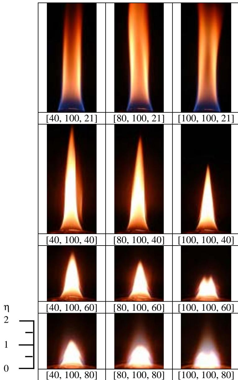
Figure 2 Direct photographs of flame appearances for different stream concentrations at constant stream velocity.
