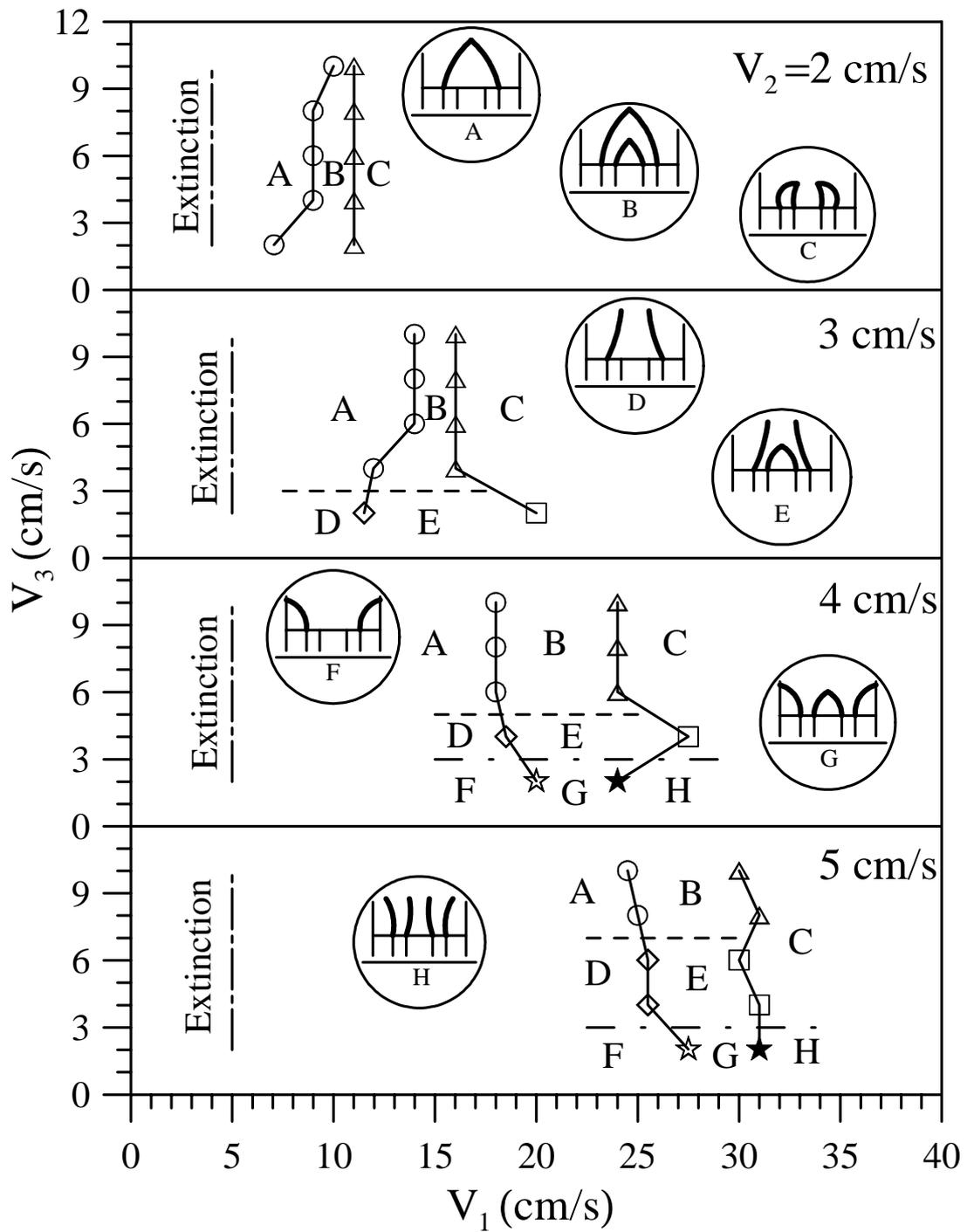
Figure 4 Map of flame configurations of tri-coaxial burner with different stream velocities.
