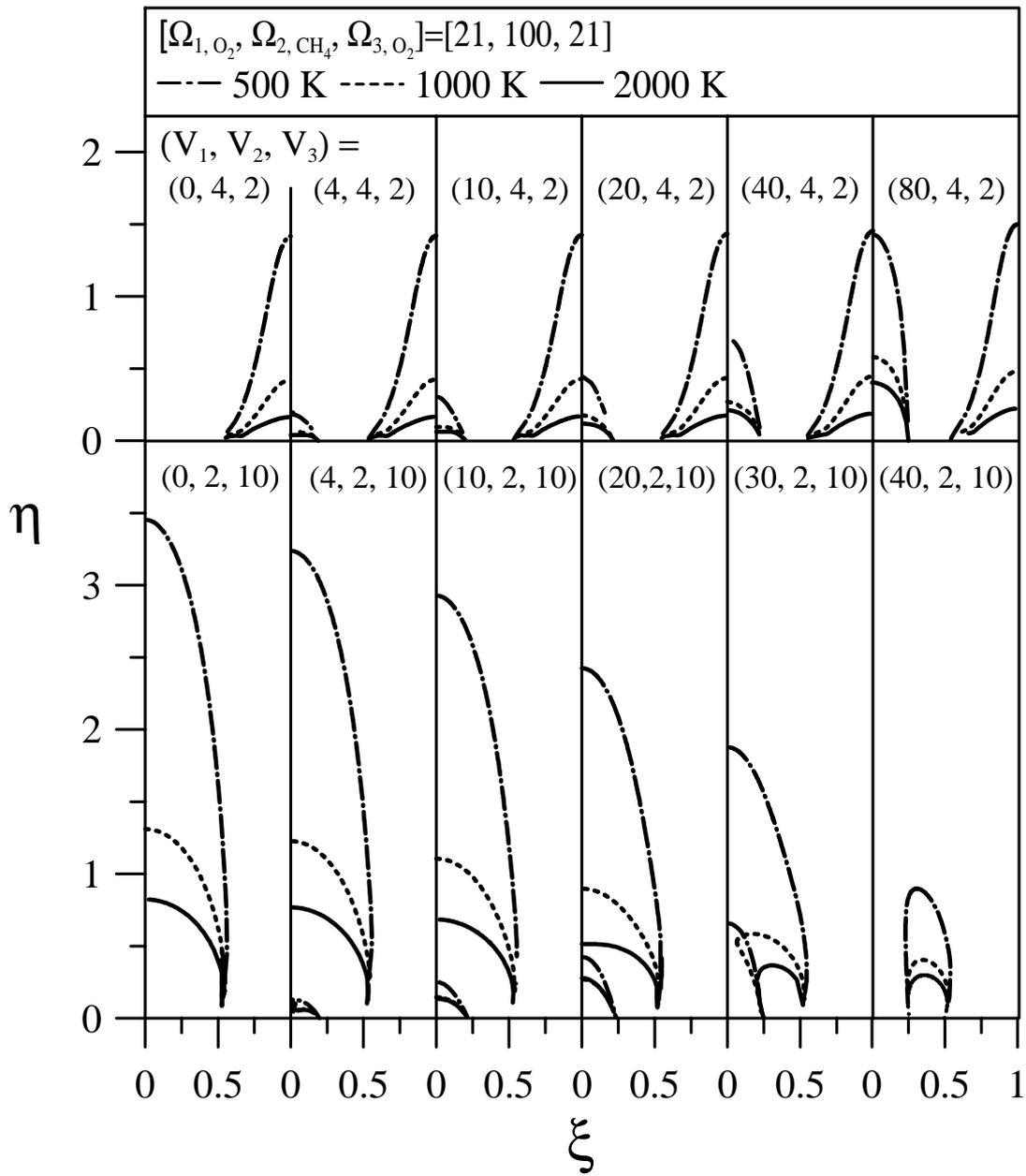
Figure 8 The prediction of flame configuration for different stream velocities at constant stream concentration.
