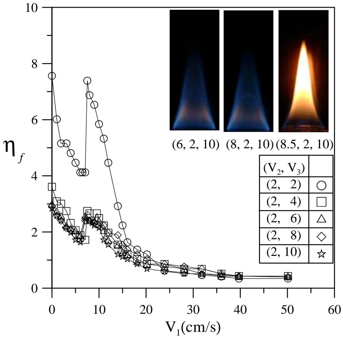
Figure 7 Effect of inner stream velocity ( $V_1$ ) on flame height.
