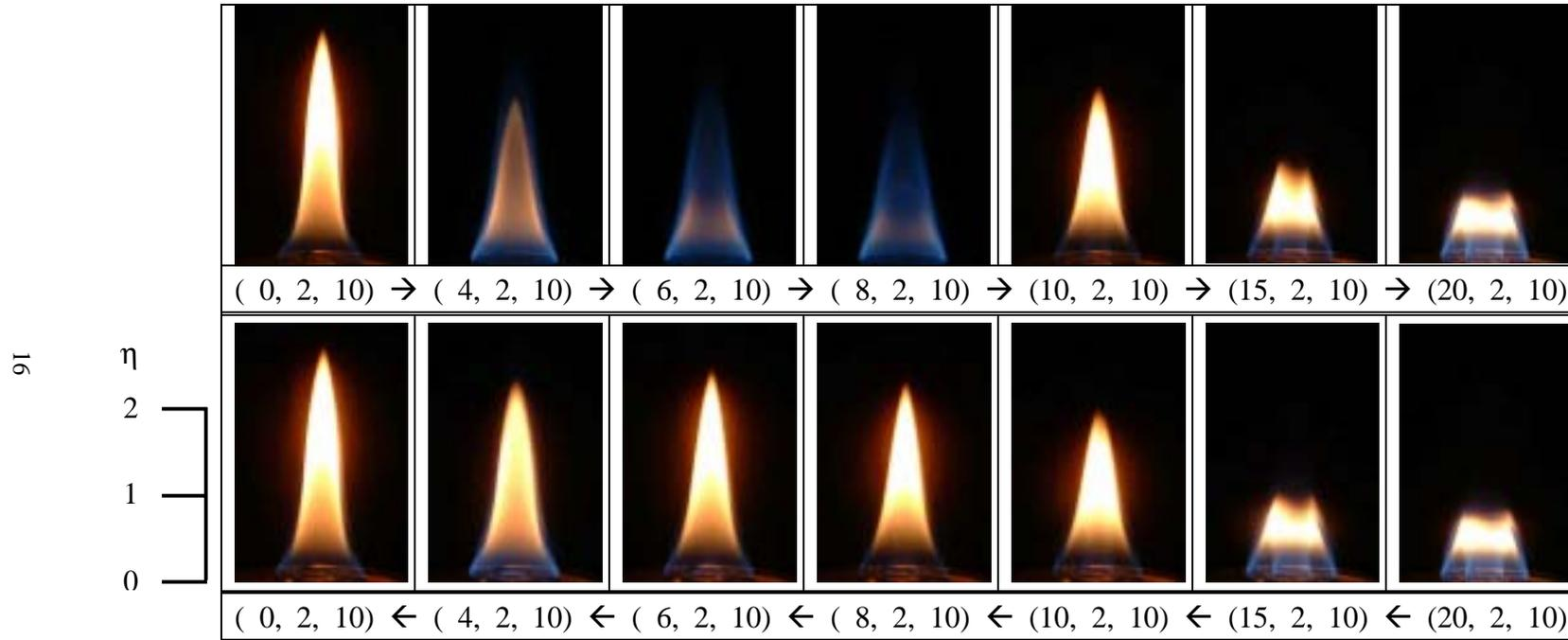
Figure 5 Direct photographs of flame transition at  $(V_2, V_3) = (2 \text{ cm/sec}, 10 \text{ cm/sec})$  by increasing or decreasing  $V_1$ .
