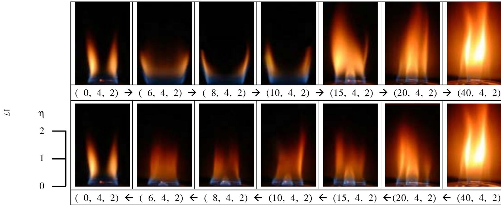
Figure 6 Direct photographs of flame transition at  $(V_2, V_3) = (4 \text{ cm/sec}, 2 \text{ cm/sec})$  by increasing or decreasing  $V_1$ .
