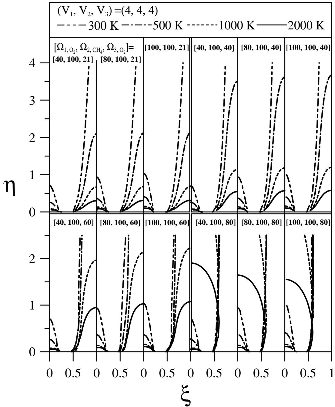
Figure 3 The prediction of flame configuration for different stream concentrations and constant stream velocity  $(V_1, V_2, V_3) = (4, 4, 4)$ .
