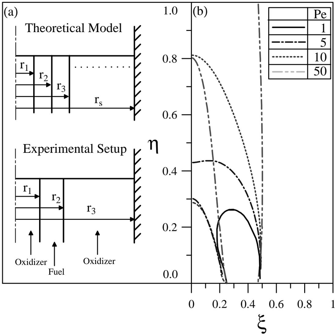
Figure 1 (a) The schematic diagrams of theoretical model and experimental setup. (b) Effect of Peclet number on flame structure and height.
