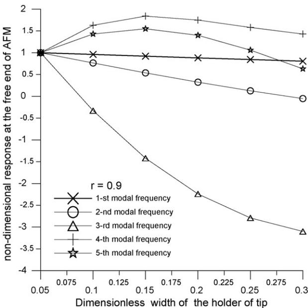
**Fig. 5 – The effect of various tip holder widths  $w$  on the response of the end point for the first five modes of  $r\omega_n$ .**
