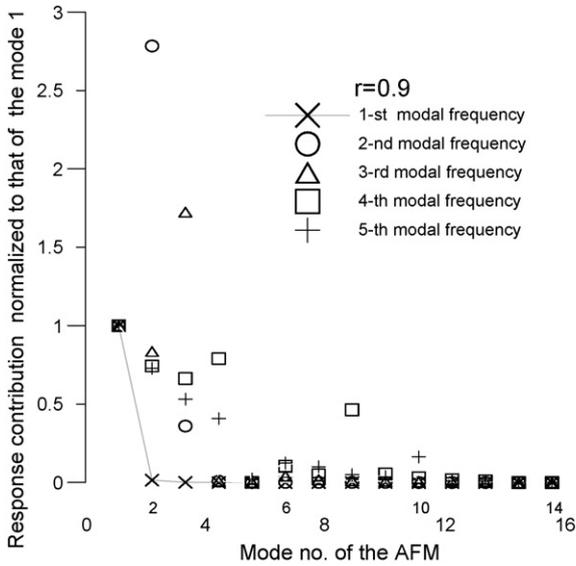
**Fig. 4 – The response contribution of each mode for an AFM cantilever subjected to various excitation frequencies with  $r=0.9$  at  $t=0.1$  s and  $x=L$ .**
