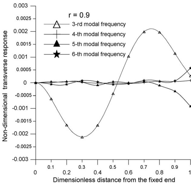
**Fig. 8 – The response for an AFM cantilever subjected to the high-order modes of  $r\omega_n$ .**
