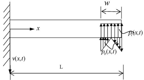
**Fig. 2 – Schematic diagram of excitations acting on the AFM.**
