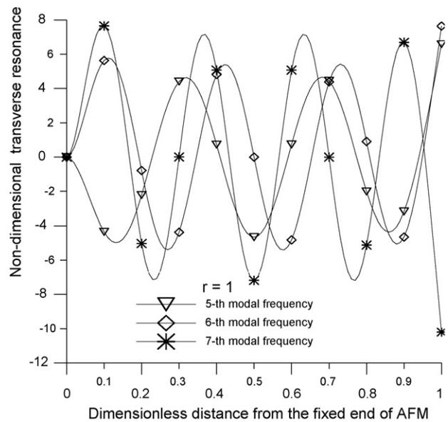
**Fig. 10 – The resonance response for an AFM cantilever subjected to harmonics cutting forces which are composed of the high-order modes of the natural frequencies.**
