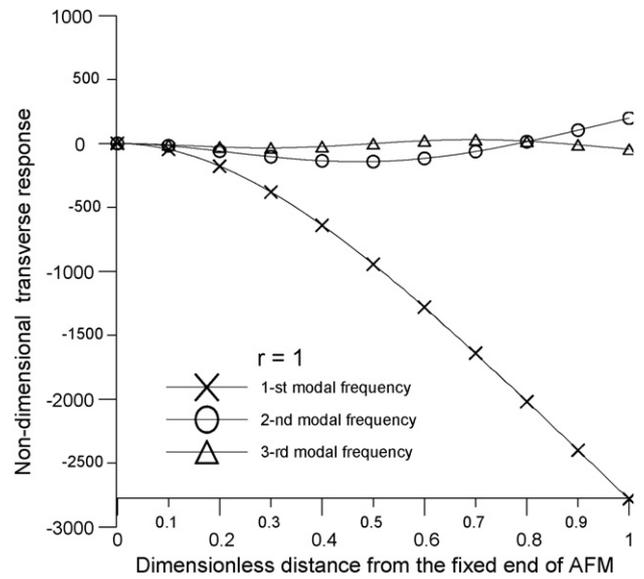
**Fig. 9 – The resonance response for an AFM cantilever subjected to harmonics cutting forces which are composed of the first three modes of the natural frequencies.**
