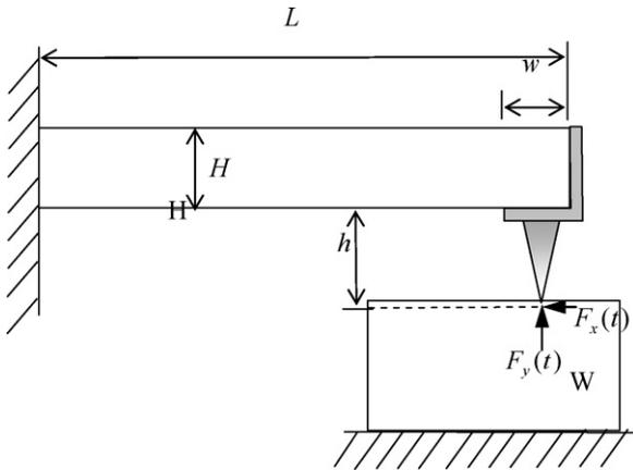
**Fig. 1 – Schematic diagram of an AFM cantilever nanomachining a sample.**
