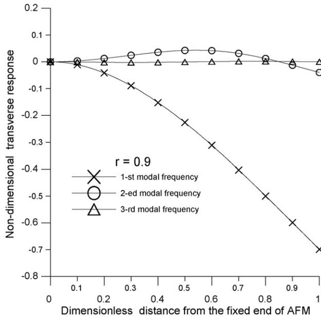
**Fig. 7 – The response for an AFM cantilever subjected to the first three modes of  $r\omega_n$ .**
