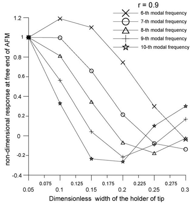
**Fig. 6 – The effect of various tip holder widths  $w$  on the response of the end point for the high-order modes of  $r\omega_n$ .**
