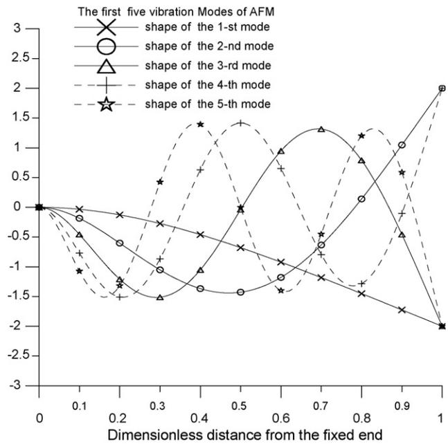
Fig. 3 – The shape of the first five vibration modes for an AFM cantilever.
