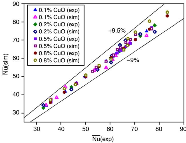
**Figure 7.** Comparison between numerical Nusselt number and experimentally measured Nusselt number at various particle volume concentrations for CuO-water nanofluids
