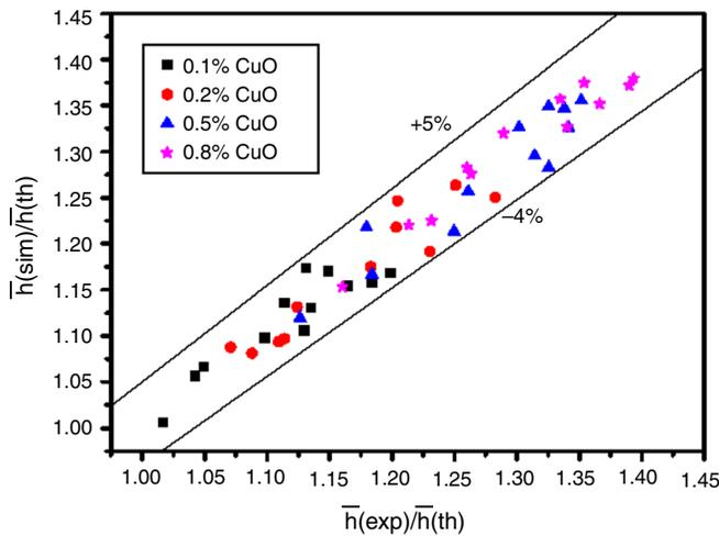
**Figure 9.** Comparison between numerical and experimental convective heat transfer coefficient to Dittus-Boelter equation at various particle volume concentrations for CuO-water nanofluids
