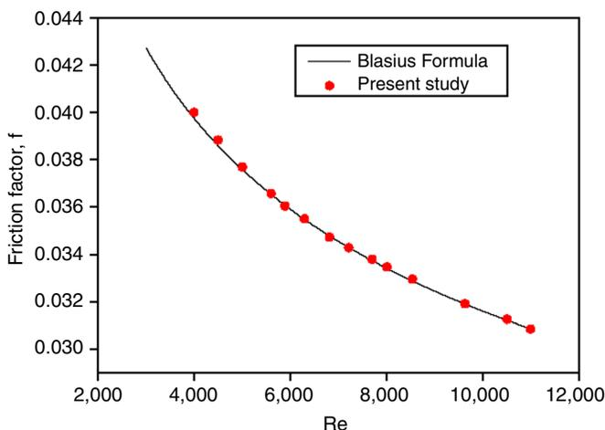
**Figure 3.** Comparison of Darcy friction factor and Blasius formula with computed values for water in turbulent regime
