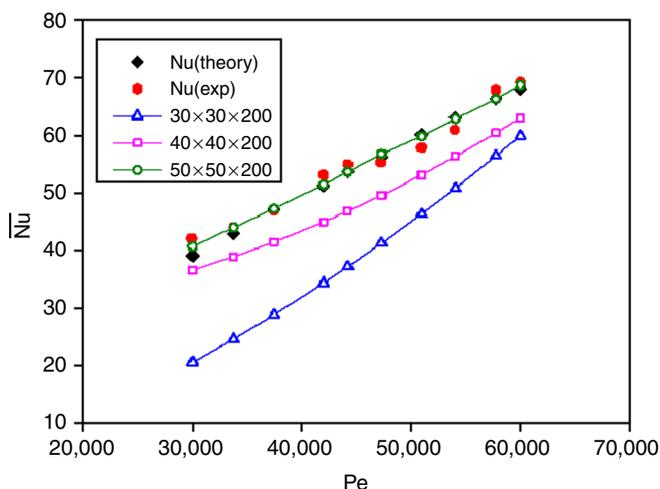
**Figure 2.** Grid sensitivity testing and comparison among numerical, theoretical, and experimental data for Nusselt number of water
