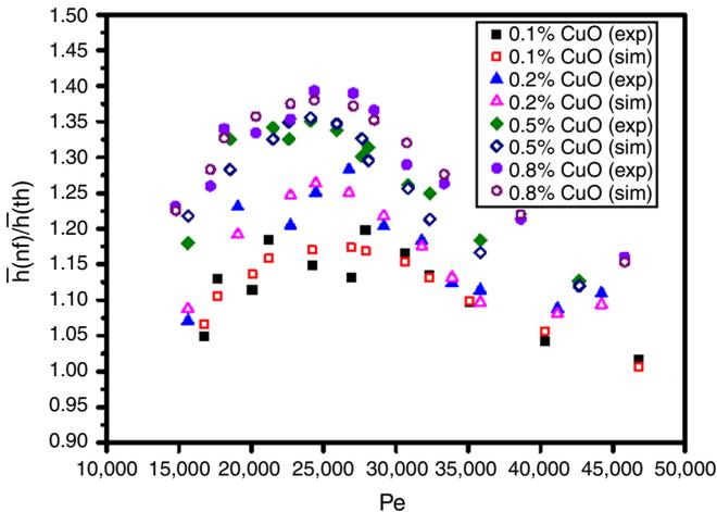
**Figure 8.** Comparison between numerical and experimental convective heat transfer coefficient to Dittus-Boelter equation vs Peclet number at various particle volume concentrations for CuO-water nanofluids
