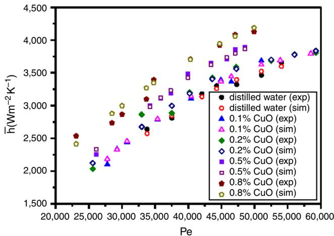
**Figure 4.** Comparison between numerical and experimental data for heat transfer coefficient vs Peclet number at various particle volume concentrations for CuO-water nanofluids
