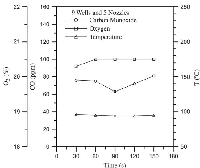
Fig. 7. The variations of CO and O<sub>2</sub> concentrations and temperature of flue gas with time as the numbers of pumping well and oil gas burner are nine and five, respectively.
