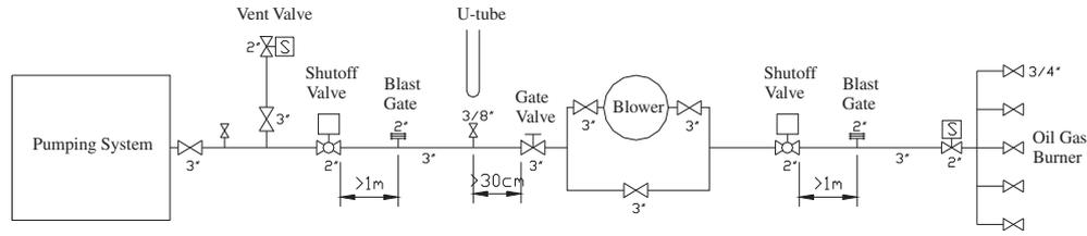
Fig. 2. Schematic of the oil gas supply and safety control system.
