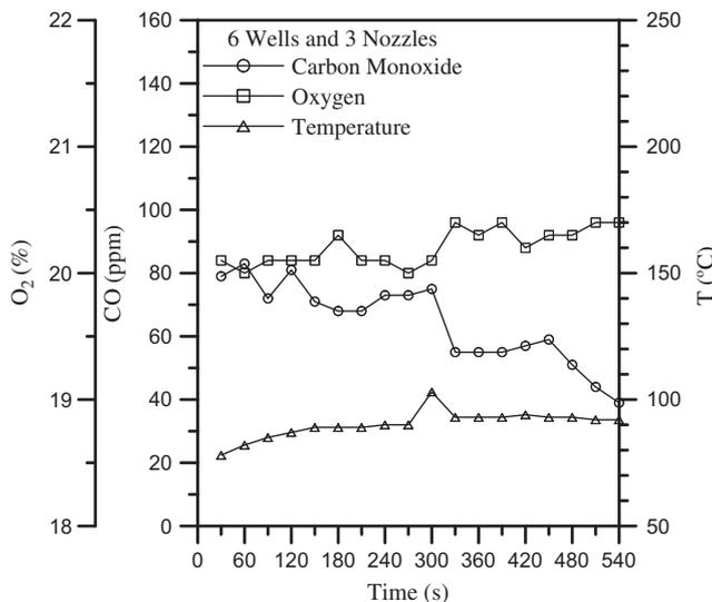
Fig. 4. The variations of CO and O<sub>2</sub> concentrations and temperature of flue gas with time as the numbers of pumping well and oil gas burner are six and three, respectively.
