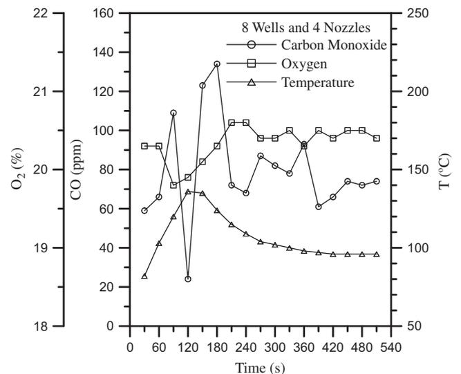
Fig. 6. The variations of CO and O<sub>2</sub> concentrations and temperature of flue gas with time as the numbers of pumping well and oil gas burner are eight and four, respectively.
