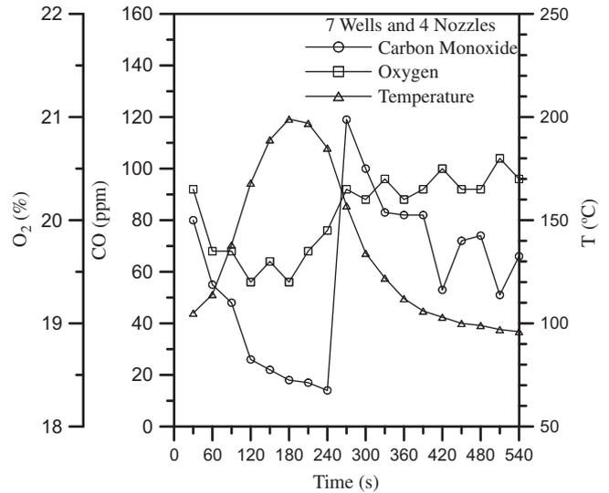
Fig. 5. The variations of CO and O<sub>2</sub> concentrations and temperature of flue gas with time as the numbers of pumping well and oil gas burner are seven and four, respectively.
