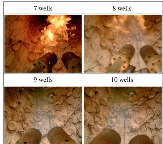
Fig. 3. The flame structures at different operating conditions.
