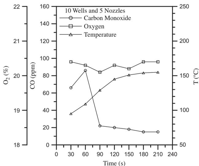
Fig. 8. The variations of CO and O<sub>2</sub> concentrations and temperature of flue gas with time as the numbers of pumping well and oil gas burner are ten and five, respectively.
