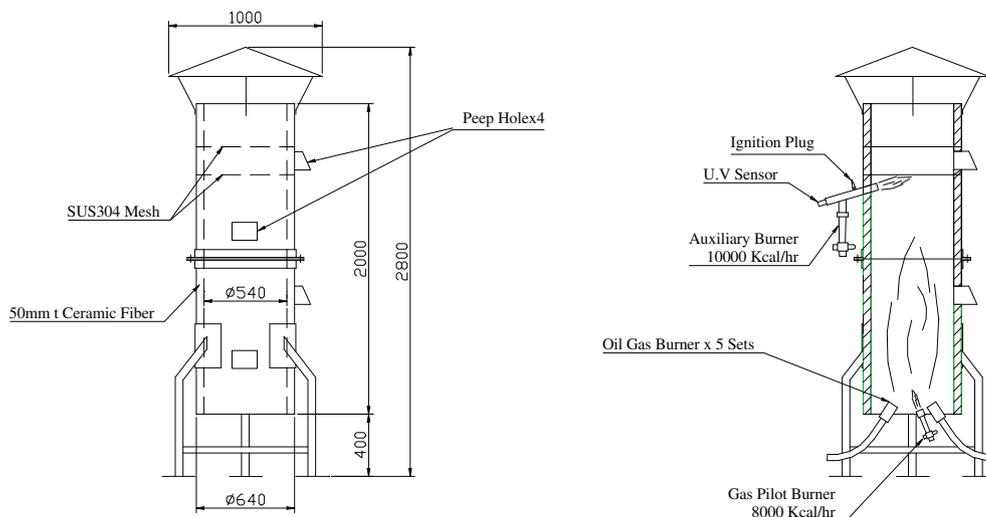
Fig. 1. Schematic of the oil incinerator.
