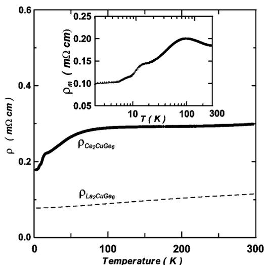
Fig. 2 Temperature dependence of electrical resistivity of  $\text{Ce}_2\text{CuGe}_6$  and  $\text{La}_2\text{CuGe}_6$  between 2 and 300 K. The inset is the magnetic resistivity  $\rho_m$  vs.  $\log(T)$
