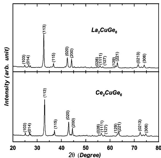
Fig. 1 X-ray diffraction patterns of  $\text{Ce}_2\text{CuGe}_6$  and  $\text{La}_2\text{CuGe}_6$
