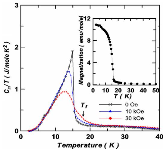
**Fig. 5** The  $C_m/T$  vs.  $T$  of  $\text{Ce}_2\text{CuGe}_6$  in 0, 10, and 30 kOe field between 2 and 40 K. The inset is the temperature dependence of magnetization  $M(T)$  of  $\text{Ce}_2\text{CuGe}_6$  between 2 and 50 K without any applied field
