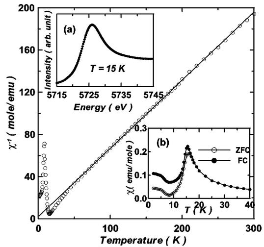
**Fig. 4** Temperature dependence of the inverse of susceptibility  $\chi_{ZFC}^{-1}$  of  $Ce_2CuGe_6$  between 1.8 and 300 K at 200-Oe field. Inset **a** is the Ce-L<sub>III</sub> edge XANES of  $Ce_2CuGe_6$  at  $T = 15$  K; inset **b** depicts  $\chi_{ZFC}(T)$  (○) and  $\chi_{FC}(T)$  (●) curves of  $Ce_2CuGe_6$  between 1.8 and 40 K
