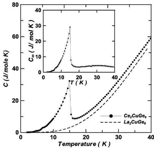
**Fig. 3** Temperature dependence of specific heat  $C(T)$  of  $Ce_2CuGe_6$  and  $La_2CuGe_6$  between 2 and 40 K. The inset plots the  $C_m(T)$  between 2 and 40 K
