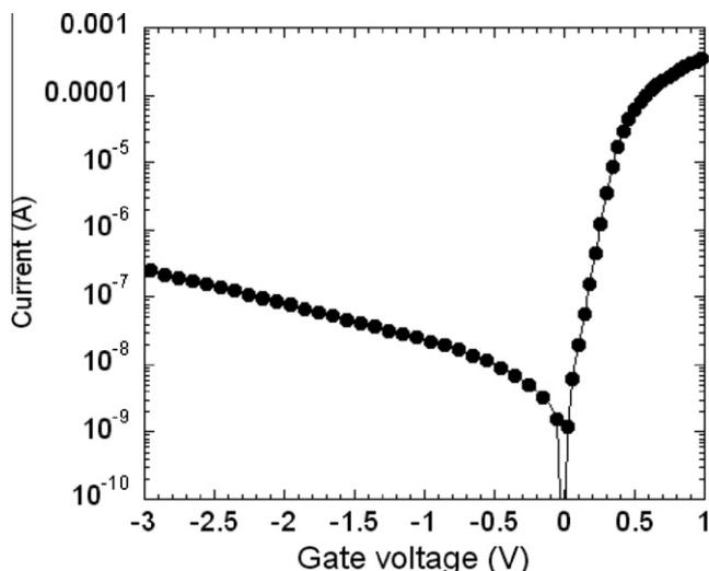
Fig. 2. The  $I$ - $V$  characteristic of the 400 °C annealed Pt/Al/n-InP diode.
