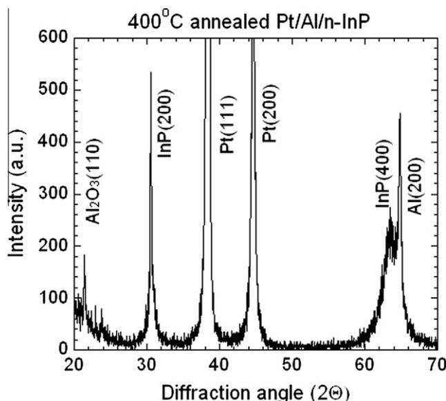
Fig. 3. The XRD analysis of the 400 °C annealed Pt/Al/n-InP diode.
