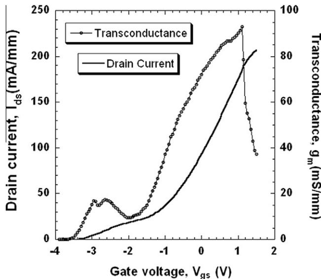
Fig. 5. The drain current and transconductance of the InP MESFET.
