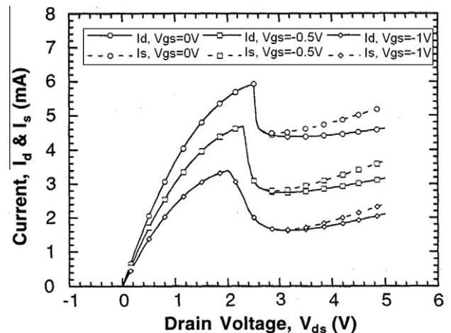
Fig. 6. The drain current ( $I_d$ ) and source current ( $I_s$ ) versus drain voltage ( $V_{ds}$ ) characteristics of the InP MESFET.
