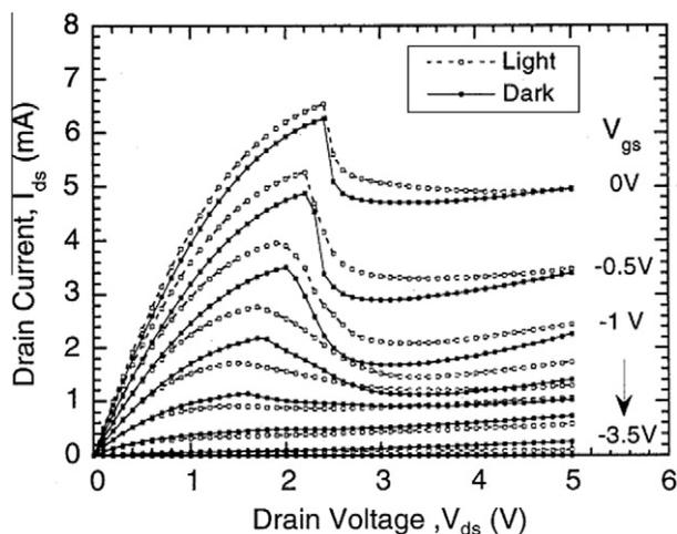
Fig. 8. The transfer characteristic of the InP MESFET with and without illumination, respectively.
