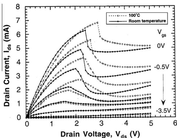
Fig. 9. The transfer characteristic of the InP MESFET which measured at room temperature and 100 °C, respectively.
