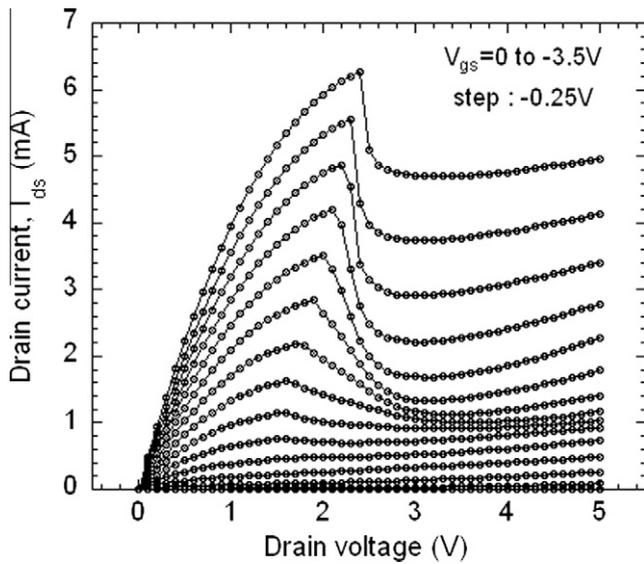
Fig. 4. The transfer characteristics of the double-metal gate, Pt/Al, InP MESFET.
