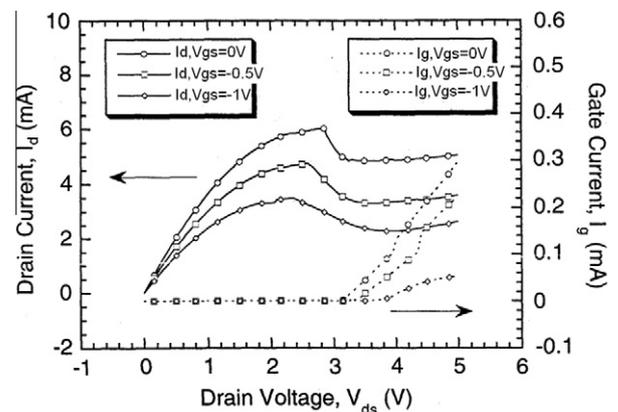
Fig. 7. The drain current ( $I_d$ ) and gate current ( $I_g$ ) versus drain voltage ( $V_{ds}$ ) characteristics of the InP MESFET.
