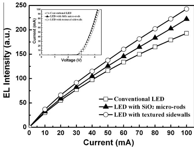
**Fig. 6.** The EL intensity as a function of injection current for the conventional LED, LED with SiO<sub>2</sub> micro-rods array and LED with textured sidewalls, respectively. The inset shows the forward *I*-*V* characteristics.
