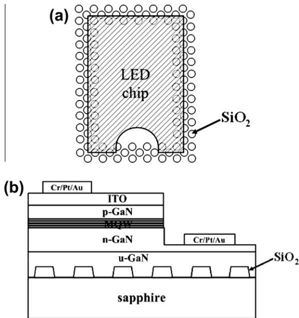
**Fig. 1.** Schematic diagram of (a) a sapphire substrate with SiO<sub>2</sub> micro-rods array at the bottom and surrounding the LED device and (b) LED structure grown on SiO<sub>2</sub> micro-rods array.
