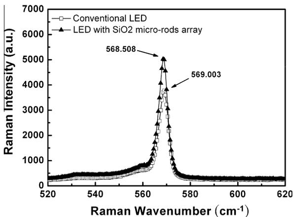
Fig. 4. Micro-Raman spectrum of the conventional LED and LED with SiO<sub>2</sub> micro-rods array.
