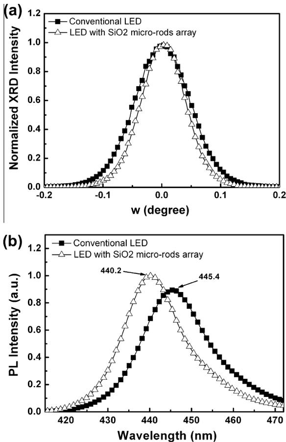
Fig. 3. (a) Normalized XRD rocking curves and (b) Normalized PL spectra measured from the conventional LED and LED with SiO<sub>2</sub> micro-rods array.
