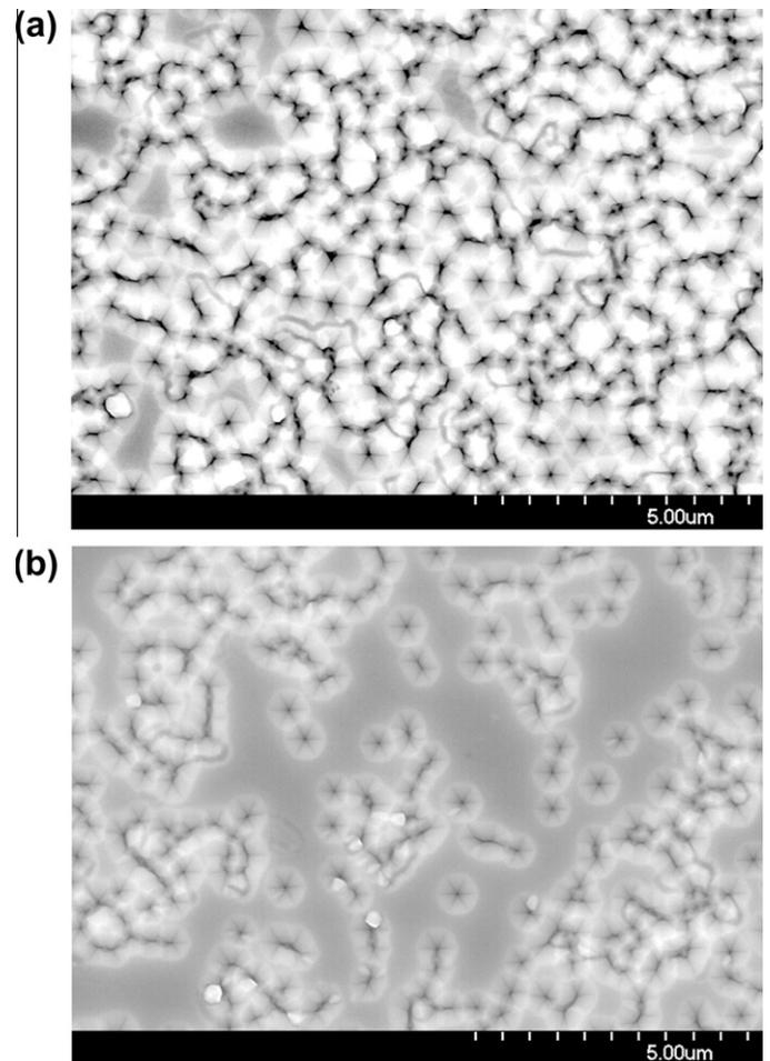
**Fig. 2.** SEM images of p-type GaN (a) grown on flat sapphire substrate and (b) grown on sapphire substrate with SiO<sub>2</sub> micro-rods array.
