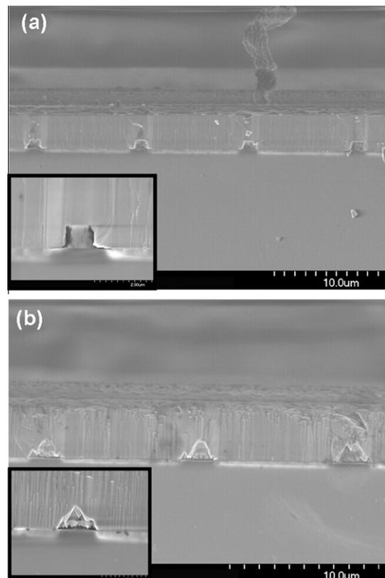
Fig. 5. Cross-sectional SEM image of (a) LED structure grown on SiO<sub>2</sub> micro-rods array and (b) after an etching time of 20 min in 5M NaOH solution.
