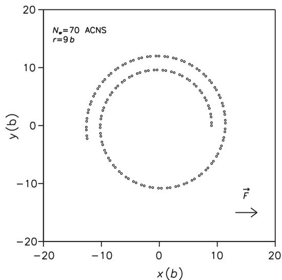
Figure 1. Cross-sectional view of a  $N_w = 70$  armchair carbon nanoscroll.
