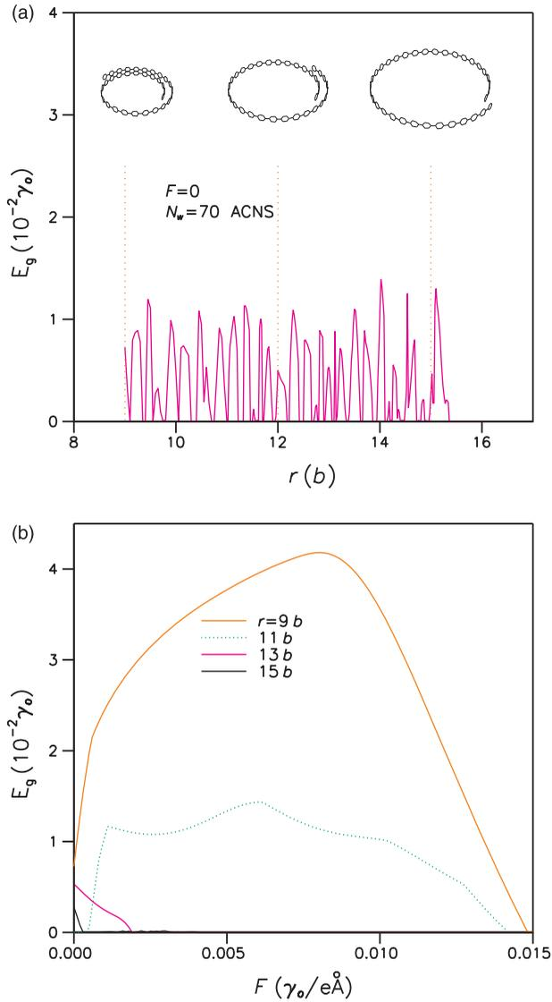
Figure 4. The energy gap of the  $N_w = 70$  ACNS versus (a)  $r$ , and (b)  $F$  with  $r = 9b, 11b, 13b$  and  $15b$ . The insets in (a) show the geometries of the  $N_w = 70$  ACNS with  $r = 9b, 12b$ , and  $15b$ . In (a), the increment step of  $r$  is  $0.05b$ .
