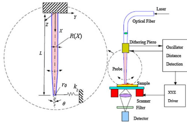
**Fig. 1.** (Color online) Schematic diagram of SNOM apparatus with a tapered probe cantilevered at one end. The interaction with the sample is modeled using the lateral spring stiffness  $k_l$ .
