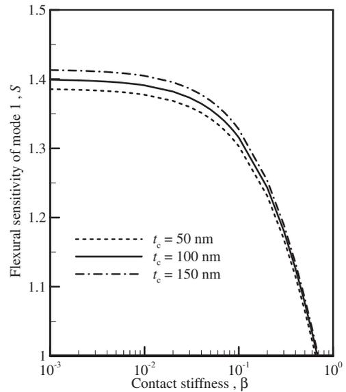
**Fig. 5.** Vibration sensitivity of mode 1 for a SNOM probe with an Al coating and a taper angle of 12° for different coating thicknesses.
