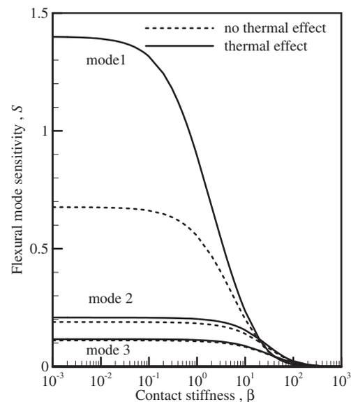
**Fig. 3.** Thermal effect on the vibration sensitivity of different modes for a SNOM probe with an Al coating of 100 nm thickness and with a taper angle of  $12^\circ$ .
