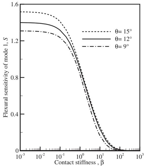
**Fig. 4.** Vibration sensitivity of mode 1 for a SNOM probe with an Al coating of 100 nm thickness for different taper angles.
