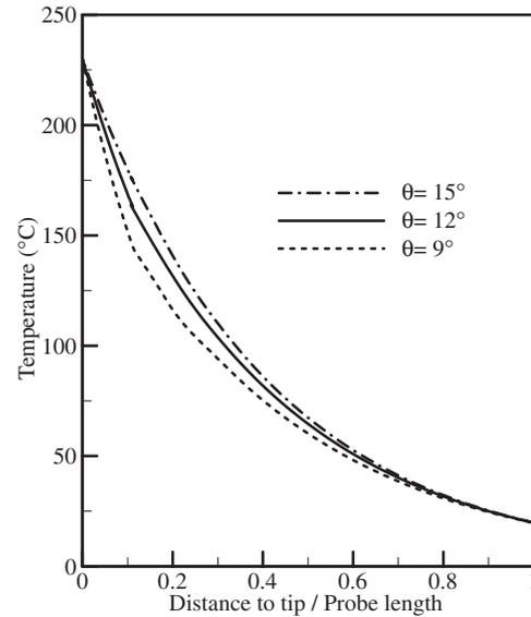
**Fig. 2.** Temperature distribution of a SNOM probe for different taper angles.
