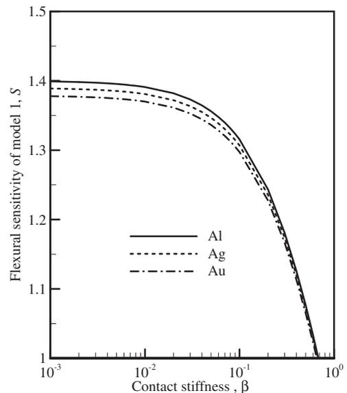
**Fig. 6.** Vibration sensitivity of mode 1 for a SNOM probe with a coating of 100 nm thickness and a taper angle of 12° for different coating materials.
