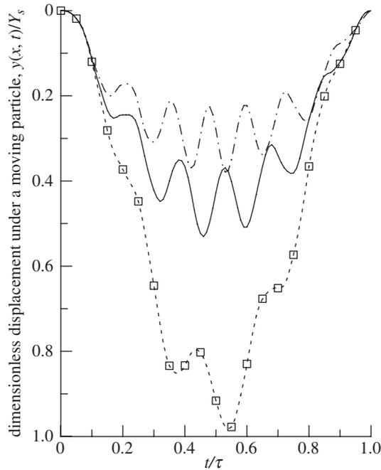
Figure 2. Dimensionless displacement of a SWCNT for nanoparticle delivery at  $\alpha = 0.1$ ,  $\rho = 0.1$  and  $k = 20$  for different dimensionless times and confined stiffnesses. Open square,  $w = 0$  (analytical); dashed line,  $w = 0$ ; solid line,  $w = 50$ ; dashed-dotted line,  $w = 100$ .
