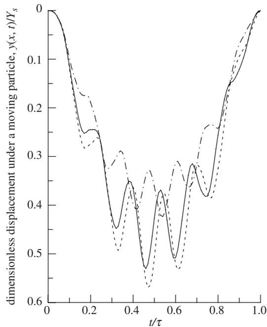
Figure 4. Dimensionless displacement of a SWCNT for nanoparticle delivery at  $\alpha = 0.1$ ,  $\rho = 0.1$  and  $w = 50$  for different dimensionless times and foundation stiffnesses. Dashed line,  $k = 0$ ; solid line,  $k = 10$ ; dashed-dotted line,  $k = 50$ .
