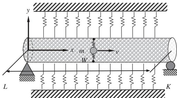
Figure 1. A nanoparticle-carrying SWCNT is assumed to be embedded in an elastic medium with two simple support ends and is described as a hollow cylindrical tube with length  $L$ .
