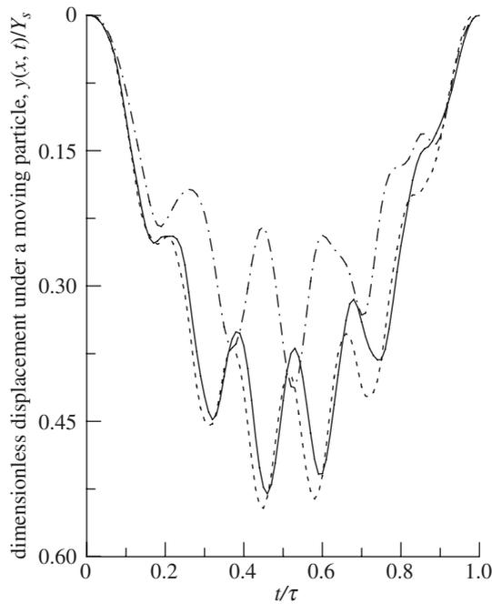
Figure 3. Dimensionless displacement of a SWCNT for nanoparticle delivery at  $\alpha = 0.1$ ,  $k = 20$  and  $w = 50$  for different dimensionless times and non-local parameters. Dashed line,  $\rho = 0$ ; solid line,  $\rho = 0.1$ ; dashed-dotted line,  $\rho = 0.3$ .
