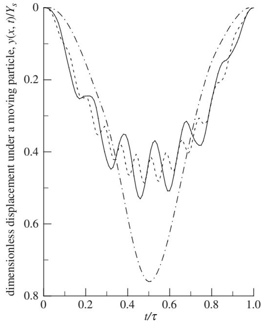
Figure 5. Dimensionless displacement of a SWCNT for nanoparticle delivery at  $k = 20$ ,  $\rho = 0.1$  and  $w = 50$  for different dimensionless times and velocity ratios of the moving nanoparticle. Dashed line,  $\alpha = 0.05$ ; solid line,  $\alpha = 0.1$ ; dashed-dotted line,  $\alpha = 0.5$ .
