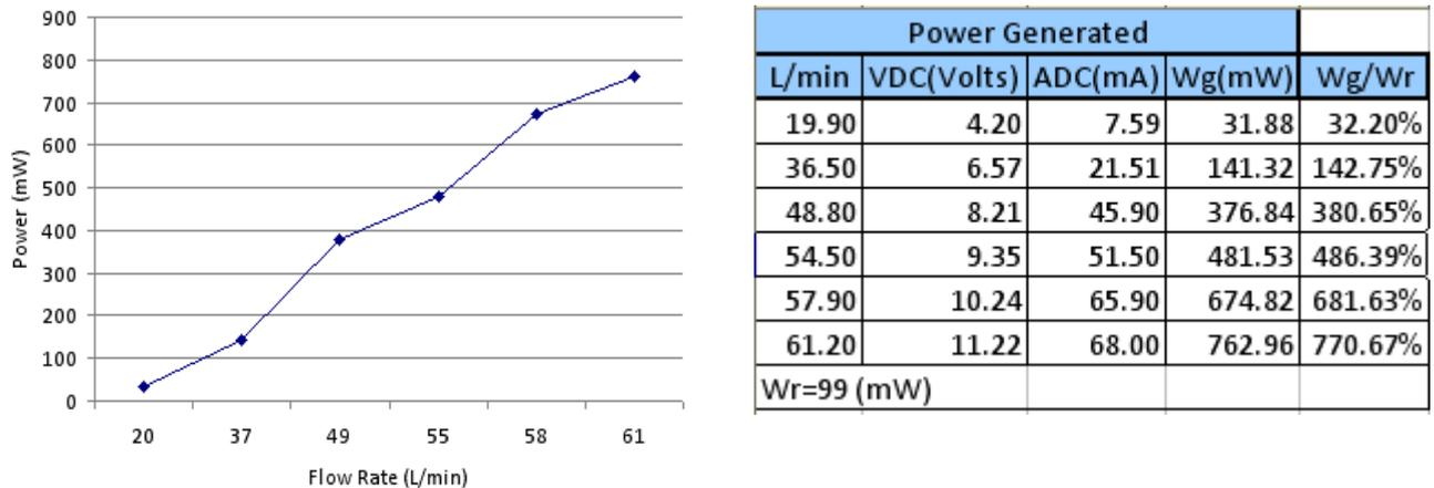
Fig. 3 Power generated vs. Flow Rate and Power required
