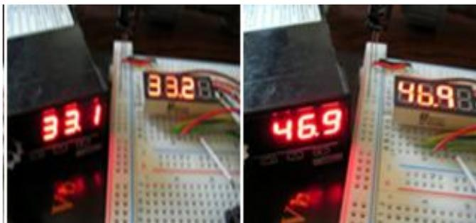
Fig. 6 Left hand side W-116 L/Min Right side SPPFM measuring system L/Min, calibrated
