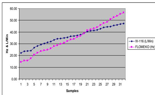
Fig. 5 SPPFM & W-116 flow measurements at different flow rates (Not calibrated)
