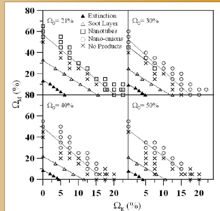
Fig. 2. Flame and synthesized products characteristics for different methane ( $\Omega_M$ ), ethylene ( $\Omega_E$ ) and oxygen ( $\Omega_O$ ) concentration.
