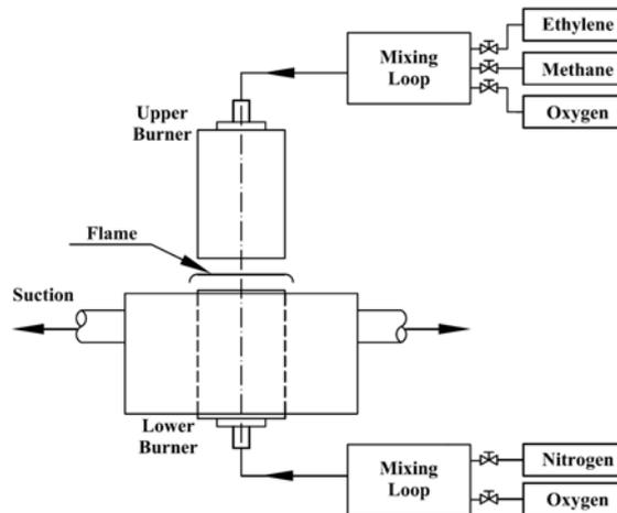
Fig. 1. Schematic of counterflow configuration.
