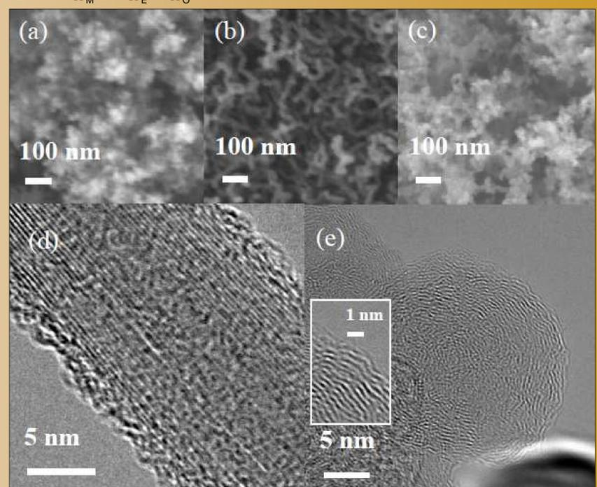
Fig. 4. SEM images of synthesized products (a) CNOs [ $\Omega_O, \Omega_E, \Omega_M$ ] = [30%, 7.5%, 30%]; (b) CNTs [ $\Omega_O, \Omega_E, \Omega_M$ ] = [30%, 7.5%, 25%]; (c) CNOs [ $\Omega_O, \Omega_E, \Omega_M$ ] = [30%, 12.5%, 25%]. HR-TEM images of (d) CNTs; (e) CNOs
