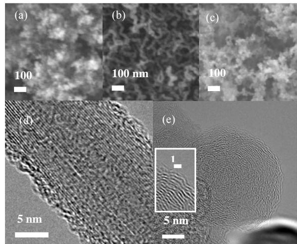
Fig. 3. SEM images of synthesized products (a) CNOs at  $[\Omega_O, \Omega_E, \Omega_M] = [30\%, 7.5\%, 30\%]$ ; (b) CNTs at  $[\Omega_O, \Omega_E, \Omega_M] = [30\%, 7.5\%, 25\%]$ ; (c) CNOs at  $[\Omega_O, \Omega_E, \Omega_M] = [30\%, 12.5\%, 25\%]$ . HR-TEM images of (d) CNTs; (e) CNOs.
