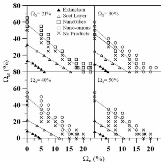
Fig. 2. Flame and synthesized products characteristics for different methane ( $\Omega_M$ ), ethylene ( $\Omega_E$ ) and oxygen ( $\Omega_O$ ) concentrations.
