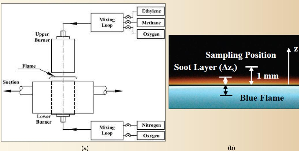
Fig. 1. (a) Experimental setup. (b) Flame structure and sampling position.
