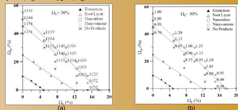
Fig. 3. (a) Temperature (in kelvin) and thickness of soot layer of sampling positions for different  $\Omega_M$  and  $\Omega_E$  at  $\Omega_O = 30\%$ .
