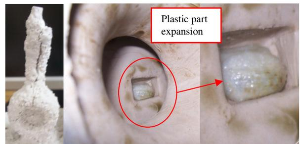
Fig.7 Plastic material flow observed after regular De-Wax process
