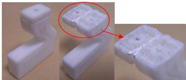
Fig. 4 Cross sectional view of the casting pattern in Fig. 2
