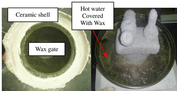
Fig. 8 Shell crack avoided by Hot-Water-De-Wax for the wax-base only
