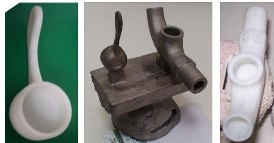
Fig. 11 Successful quick-cast metal pieces with thin walls
