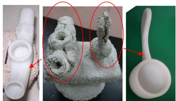
Fig. 6 Shell crack after regular De-Wax process up to 180 °C
