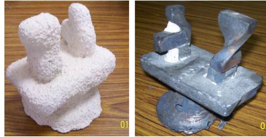
Fig. 5 Ceramic shell and steel parts with gate and feeding base
