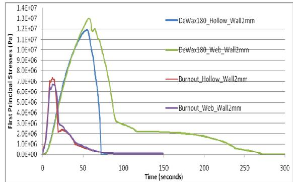
Fig. 15 Shell stresses during de-waxing and burnout (2 mm Wall)
