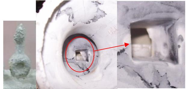
Fig. 10 Very clean ABS burn-out under 1100°C without shell crack
