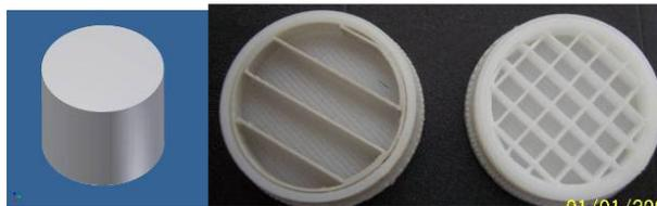
Fig. 3 Cross sections of a cylinder (30x20mm)
