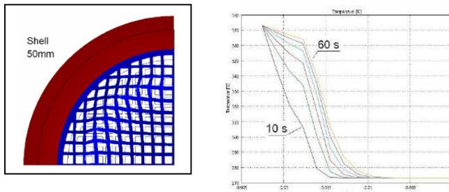
Fig. 13 Temperature propagation towards inner structure
