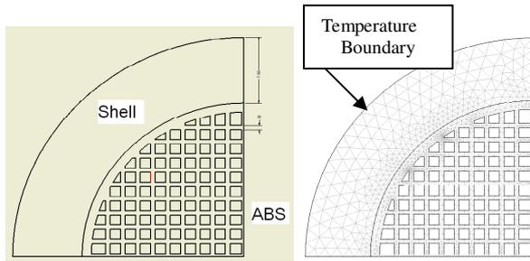
Fig.12 Physical model and mesh situation from COMSOL Multi-physics<sup>R</sup>
