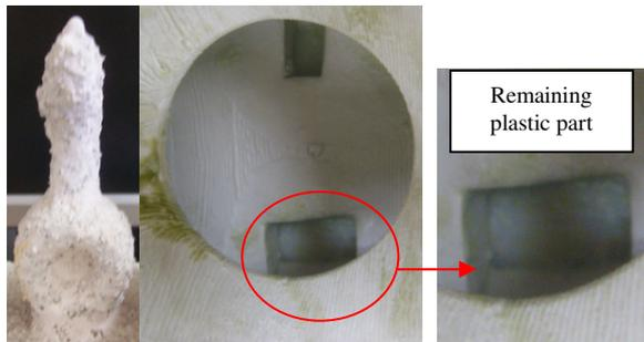
Fig. 9 ABS RP part remains in original shape after Hot-Water-De-Wax
