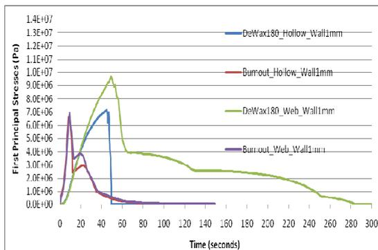
Fig. 14 Shell stresses during de-waxing and Burnout (1 mm Wall)
