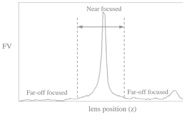
Fig. 2 FV variation for a large depth of lens displacement.
