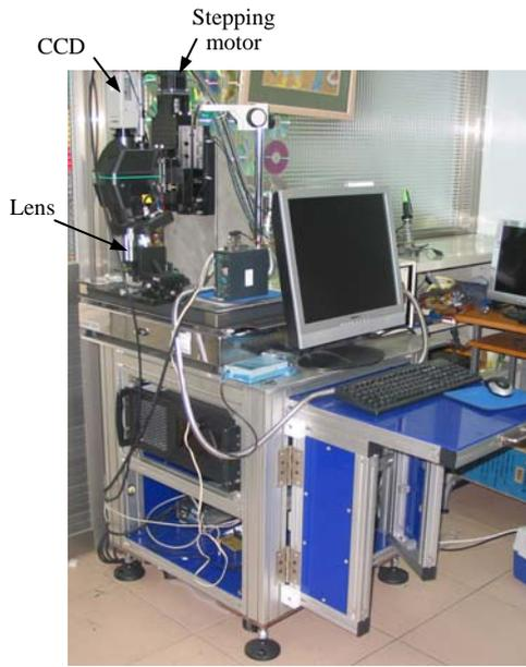
Fig. 8 Photo of the AF system setup for this study.
