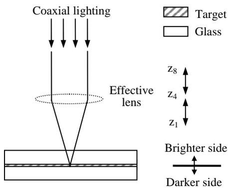
Fig. 4 Schematic of LCD panel under focusing.
