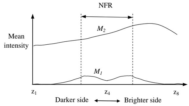
Fig. 5 Two optical mechanisms of the measure  $M_{int}$ .
