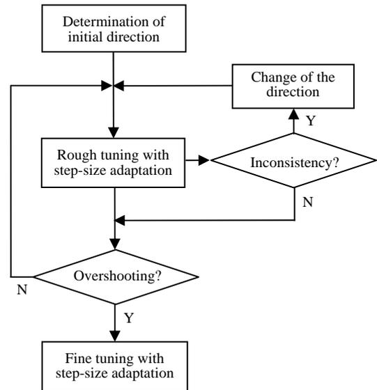
Fig. 7 Flowchart of the proposed focusing control algorithm.
