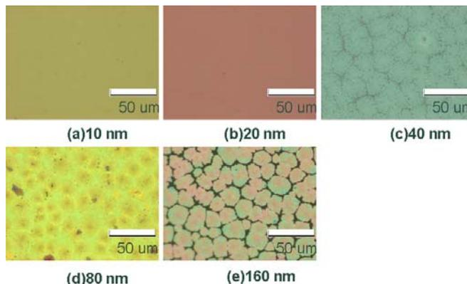
Figure 2. OM top view images of poly silicon films with different aluminum thickness of (a)10, (b)20, (c)40, (d)80, and (e)160 nm.
