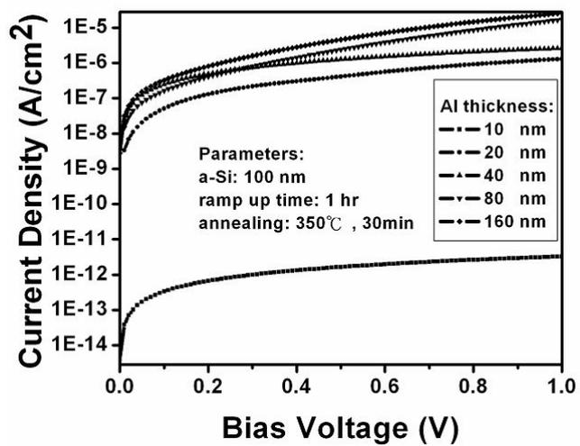
Figure 5. Leakage current density of specimens vs bias voltage under different aluminum thicknesses.
