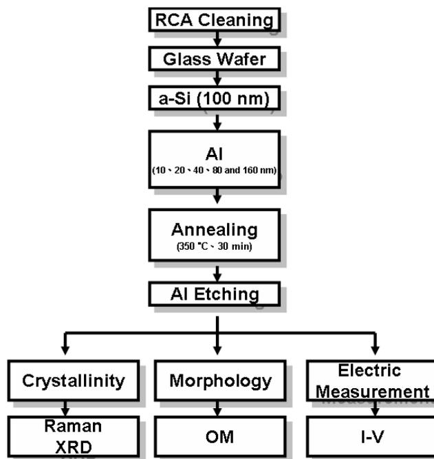
Figure 1. Process flow of the AIC method
