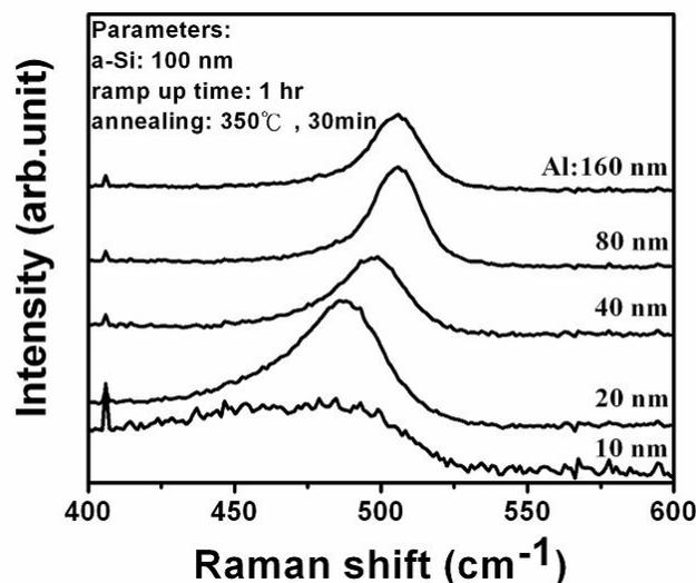
Figure 3. Raman spectra of poly silicon films with five different aluminum thicknesses.
