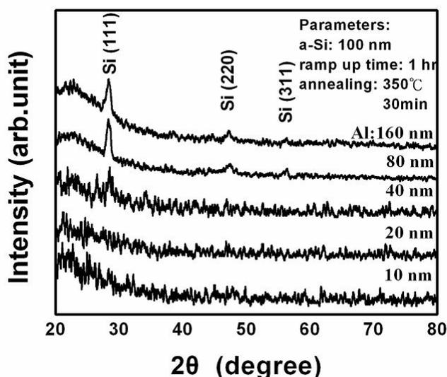
Figure 4. XRD spectra of poly silicon films with five different aluminum thicknesses.
