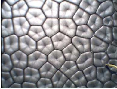
Fig.3 Honeycomb-like cell pattern observed in Bénard convection.
