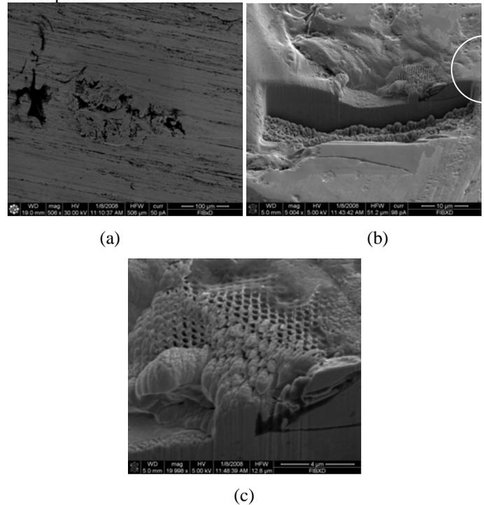
Fig.2 FIB images of the Bénard cell-like worn surface type. (a) The scuffed cavity located at the worn spot; (b) FIB milling technique applied inside the worn spot; (c) Magnification of the Bénard cell-like worn surface shown in (b).
