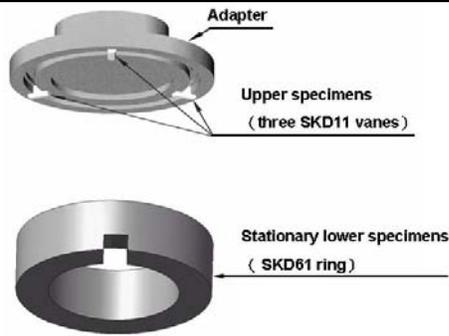
Fig.1 3D illustrations of the vanes-on-ring test specimens and adapter
