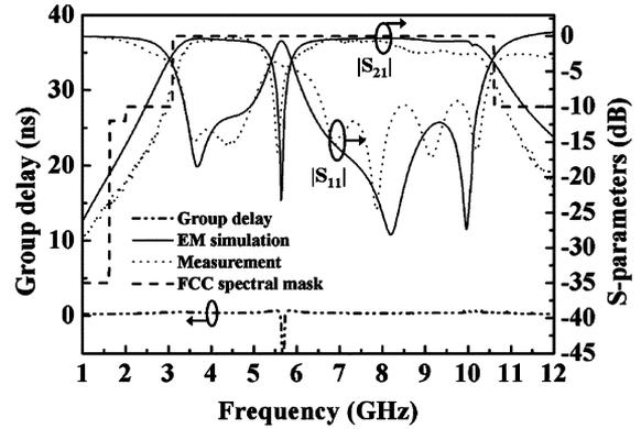
Fig. 5. Photograph and measured results of the fabricated BPF.  $S_1 = S_2 = W_1 = 0.1 \text{ mm}$  and  $W_2 = 0.3 \text{ mm}$ .
