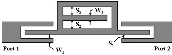
Fig. 1. Configuration of the UWB BPF with the embedded open-circuited stub structure.
