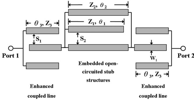
Fig. 2. Equivalent transmission line model of the proposed UWB filter.
