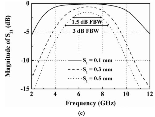
Fig. 3. (a) Transmission line model, (b) the real part of the image impedance with  $c$  and  $p$  mode and (c) EM simulated frequency response of the asymmetric coupled line under different coupling gap  $S_1$ .
