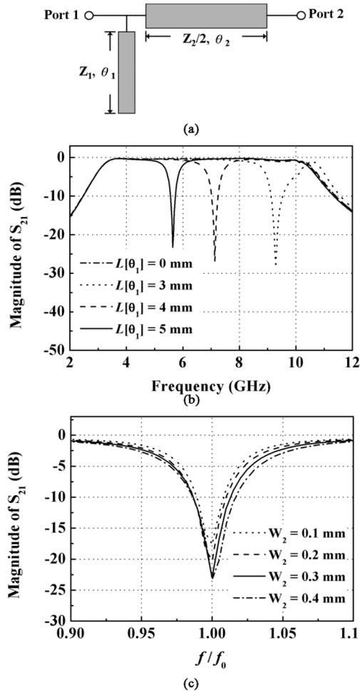
Fig. 4. (a) Equivalent circuit model of the embedded open-circuited stub in the MMR, and simulated frequency response with tuning (a) the physical length  $L$  and (b) the width  $W_2$  of the embedded open-circuited stub.
